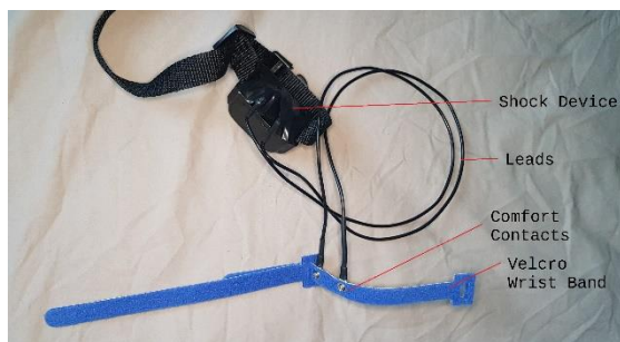
Figure 1: Annotated image of the electric shock device modified to be more comfortable.
